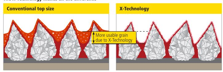
• On conventional abrasives the space between the grain is filled with top size which leads to less usable grain and therefore reduced lifetime of the disc.
