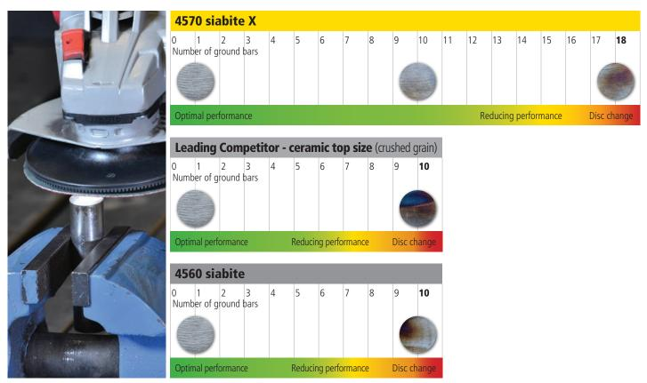
\* Tested on stainless steel bars Ø 20mm, # 60, 10 sec. on each bar. Manual test. Turbo Backing Pad II. 1100W angle grinder.
