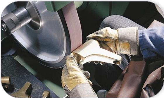
2946 siatur jj is an all-purpose product suitable for the surface treatment of profiles and contoured steel surfaces, hard to grind metals and non-ferrous metals using stationary or manually-operated abrasive belt machines – it delivers impressive results every step of the way from deburring to the perfect finish.
