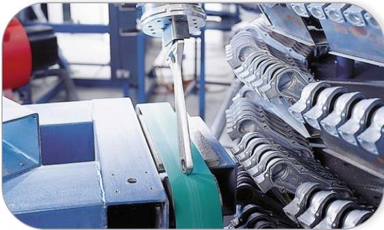
The special 2803 siaron y series is designed for high-alloy steels and other hard to grind metals, it comes into its own in applications such as the industrial surface treatment of weld seams and transitions as well as the removal of mill scale – thanks to a combination of high stock removal rates, low surface pressure and extremely long life.
