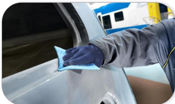
With 9215 Flat Pad, work such as sanding, fine sanding, matting and preparation for polishing is particularly easy. High flexibility for optimal adaptation to contours, curves and profiles - and thus enables high-quality, uniform sanding pattern.
