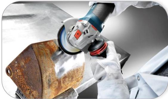
6300 siastrip for unalloyed and low-alloyed steel leaves nothing to be desired in terms of removal rates and product life, and also has the advantage of low clogging.
