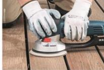
☐ For a finer surface finish, perform an additional sanding step
