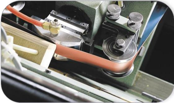
Designed for profile sanding of radii between 5–10 mm, 2936 siatur jj achieves a high level of dimensional accuracy during profile belt sanding applications and delivers perfect results when sanding profiled work pieces.
