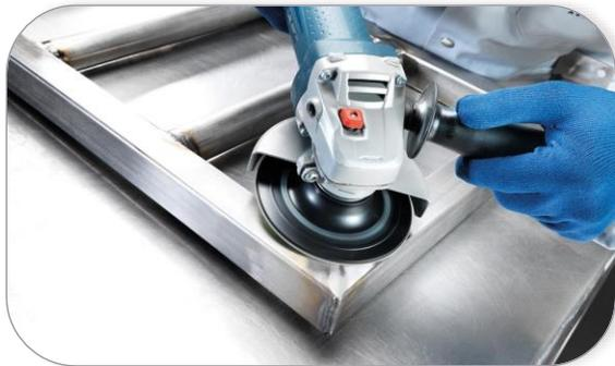
As specialist products for high-alloy steels, 4815 siacut fibre discs are suitable for a variety of applications: from general dressing work, deburring and edge chamfering through to the surface treatment of bronze ship propellers. Active cooling ingredients keep discolouration to a minimum.
