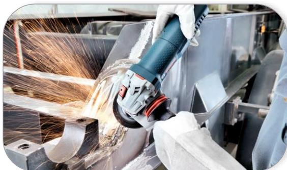
The 4961 sialoX fibre disc series with its excellent price/performance ratio is suitable for all unalloyed steels, low-alloy steels and non-ferrous metals.
