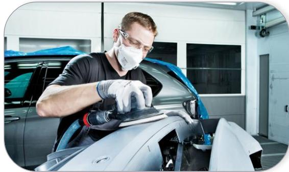
The versatile all-round product 1950 siaspeed is specially designed for high stock removal rates, perfect surface quality and long life in applications such as the surface treatment of body filler, primer filler, lacquers and paints.
