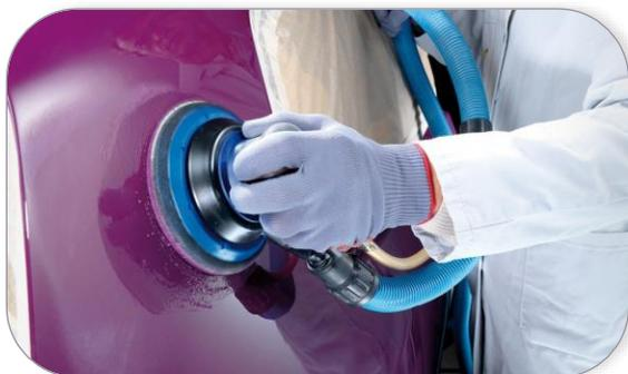
Whether it's scuffing, fine sanding or preparation for polishing – the improved technology of 7940 siaair is the key to a perfect finish in damp sanding applications.
