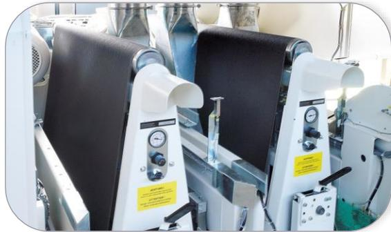
A specialist abrasive for keying MDF, HDF and chipboard, 1749 siaral f not only has a long lifetime, it also produces a high-quality surface finish.
