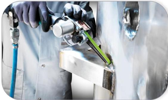
2511 siabite abrasive belts are designed especially for power file sanders and provide maximum efficiency on high-alloy steel and other hard to grind metals thanks to the self-sharpening effect of the ceramic grit.
