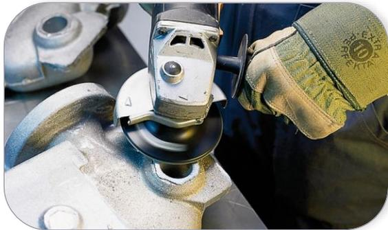
Specially designed for applications involving steel and non-ferrous metals, 4819 siaron 8 fibre discs achieve, among other things, high stock removal rates and have a long life.
