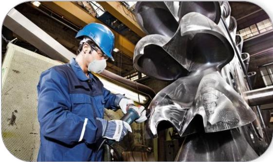
Thanks to innovative X-Technology, 4570 siabite fibre discs bring you considerably cooler grinding with a long service life and a consistent cutting performance on stainless steel and mild steel. With new and unique X-Technology, an active cooling aid is applied directly to the top level, which enhances cooling and minimises discolouration.
