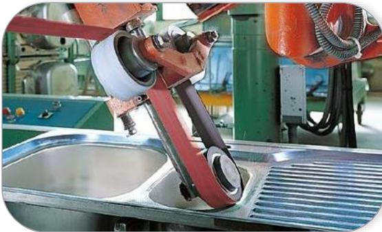
Thanks to the triangular shape of the ceramic grain, the strong polyester backing and the cooling agent, the 2582 siaramic abrasive belt offers the highest removal rate and longest lifetime on stainless steel and other metals.
