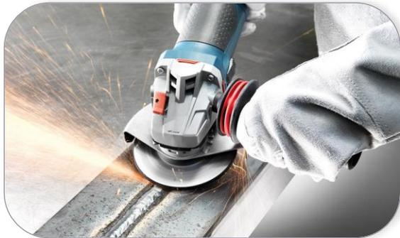
The hard grinding discs of the special 8933 siagrind series excel in a variety of metal applications and make for robust and efficient tools thanks to features such as high removal rates at low surface pressure and long life.
