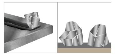
**Conventional, crushed ceramic grain** Conventional (crushed) grain is irregular and blocky in shape which results in a "ploughing" action and generates unwanted heat when grinding.
