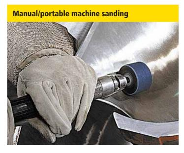
For treating surfaces using an angle grinder, a die grinder, power file or orbital sander, or by manual sanding.
